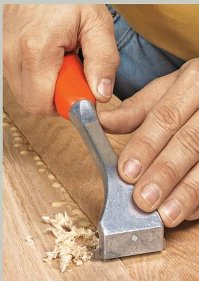
Let squeeze-out from polyurethane glue harden completely before trying to remove it. Then scrape it off using a sharp paint scraper. A carbide scraper works especially well.
